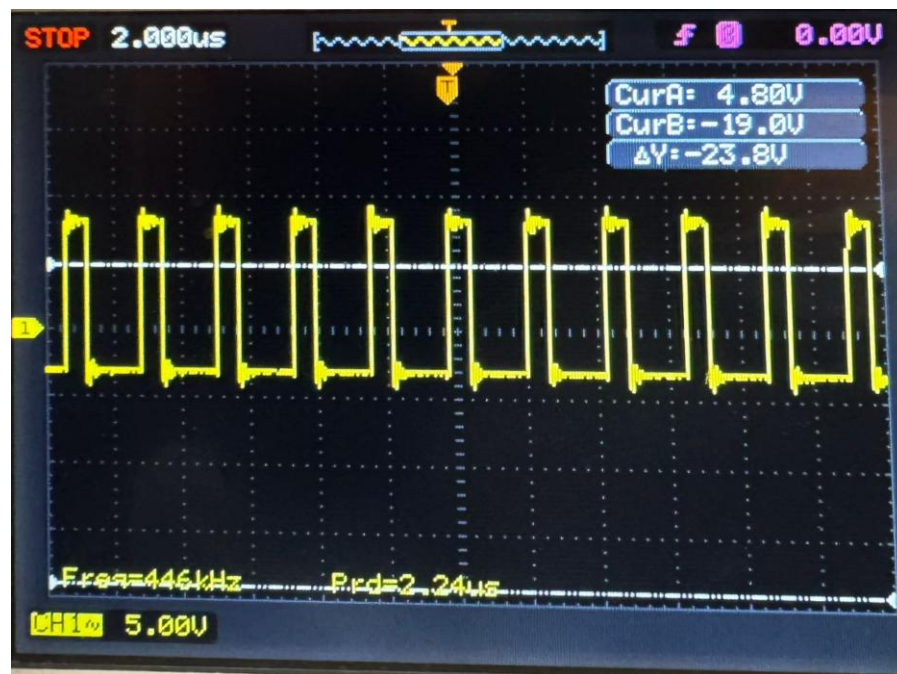
Current load = 1A Duty cycle ≈ 27.3%
