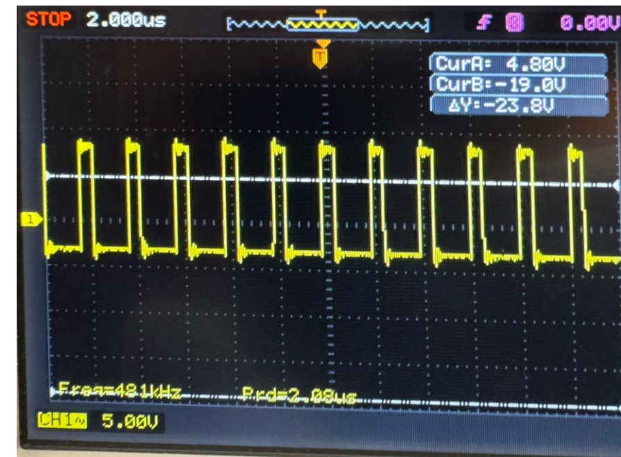
Current load = 5A Duty cycle ≈ 28.6%
