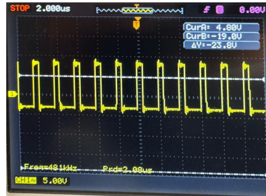
Current load = 5A Duty cycle \approx 28.6%
