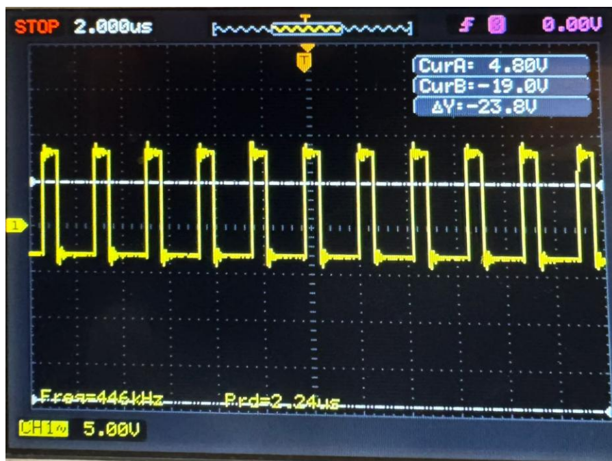
Current load = 1A Duty cycle \approx 27.3%
